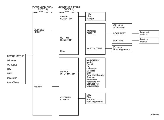
Figure 4-3. Menu Tree for HART/AMS on the Two-Wire In Situ Oxygen Analyzer (Sheet 3 of 3)
